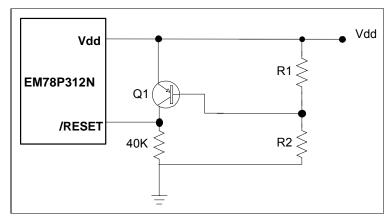
Fig. 5-36 Residue Voltage Protection Circuit 2
